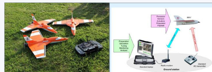
Figure 3: The SUMO model frame is small, with wingspan of 0.8 meters (left, photo J. Reuder). The operational weight of the SUMO is less than 0.6 kg and it can reach altitude of more than 4000 m.a.g.l. Right panel shows a schematic of how the SUMO is operated; a combination of a ground station (the paparazzi autopilot) and remote (manual) control.
