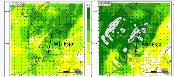
Figure 4: Simulated and observed (red flags) surface winds at 19 July 2009 at 15:00 UTC. The model simulates a sea-breeze (left) that is not seen in observations. When using five SUMO profiles, taken in the lee of Mt. Esja, to nudge the simulation, the flow structure becomes in much better agreement with available observations (right).
